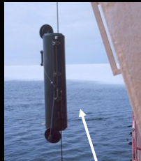
A Nansen bottle is a device for obtaining samples of seawater at a specific depth. It was designed in 1910 by the early 20th-century explorer and oceanographer Fridtjof Nansen and further developed by Shale Niskin ( Wikipedia.com )
